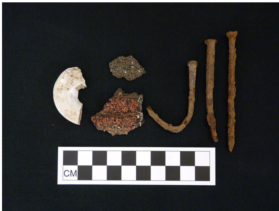
Image 15: Structural: wrought nail, machine cut nail and wire nail. From fill deposits: porcelain insulator, asphalt shingles.
